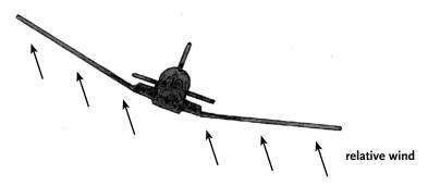
Because of the dihedral angle of the wings, the relative wind (created by movement of an airfoil through the air) will strike the lower wing at a greater angle of attack than the upper wing, producing more lift in the lower wing and helping return the aircraft to a stable lateral position.
