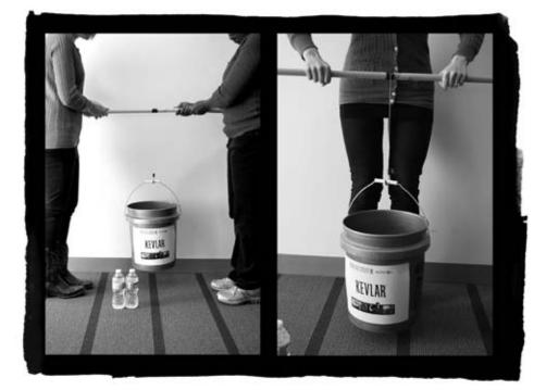
**6.** Note: Due to the very low tensile strength of the cotton, the line may break immediately, under just the weight of the bucket. After each line breaks, the water bottles from that bucket can be used to continue the test. The likely outcome of the test is shown at right.
