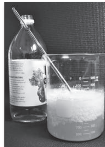
When vinegar is added to milk, a bioplastic forms.
